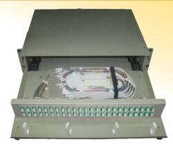
Fibre Termination Units are used for termination and management of Fibre backbone and equipment cables in Central Office and bulk fibre distribution systems. It serves as the interface between field cables and equipments. Cables may be terminated direct or after splicing. Provision has been made for internal fibre management by cable spooling with minimum bend radius and stackable splice trays. Rack mounted versions are designed for flange mounting on 19 inch racks.
